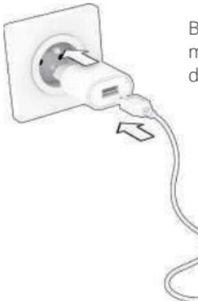
Before first use, please fully charge the solar module for at least 8 hours using the charging dock and USB-A cable.
